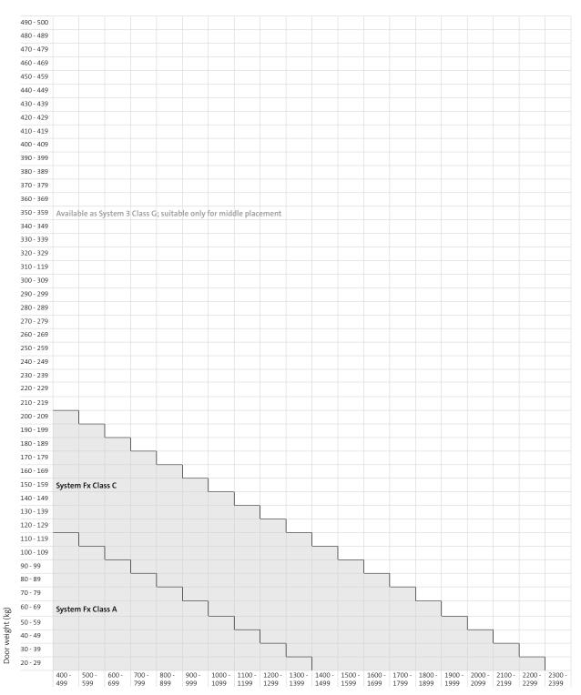
Distance of pivot point to the far edge of the door (mm)
